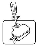
5. Replace the battery cover and tighten the screw to secure.
